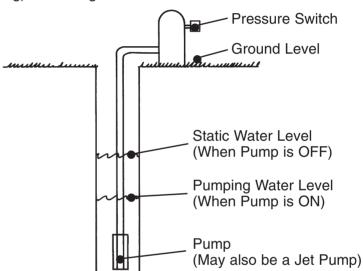
**CAUTION:** If the pumping level used to calculate pipe requirements for a well is substantially above the bottom and the pumping level drops due to drought or other conditions, the pressure rating of the pipe could be exceeded.
