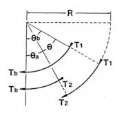
$$\begin{split} \Theta &= \Theta_{b} - \Theta_{a} \\ T_{b} &= T_{1} \epsilon^{K\Theta} b - \frac{WR}{1+K^{2}} \left[ 2K \epsilon^{K\Theta} b \sin \Theta_{b} + (1-K^{2}) \left( 1 - \epsilon^{K\Theta} b \cos \Theta_{b} \right) \right] \\ T_{2} &= \left( \frac{T_{b} + \frac{WR}{1+K^{2}} \left[ 2K \epsilon^{K\Theta} a \sin \Theta_{a} + (1-K^{2}) \left( 1 - \epsilon^{K\Theta} a \cos \Theta_{a} \right) \right]}{\epsilon^{K\Theta} a} \right) \end{split}$$
