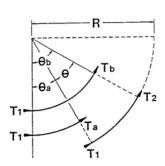
$$\begin{split} \Theta &= \Theta_{b} - \Theta_{a} \\ T_{a} &= T_{1} \varepsilon^{K\Theta} a - \frac{WR}{1 + K^{2}} \left[ 2K \sin\Theta_{a} - (1 - K^{2}) \left( \varepsilon^{K\Theta} a - \cos\Theta_{a} \right) \right] \\ T_{b} &= T_{1} \varepsilon^{K\Theta} b - \frac{WR}{1 + K^{2}} \left[ 2K \sin\Theta_{b} - (1 - K^{2}) \left( \varepsilon^{K\Theta} b - \cos\Theta_{b} \right) \right] \\ T_{2} &= T_{b} - T_{a} + T_{1} \end{split}$$
