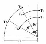
$$\begin{split} \Theta &= \Theta_{b}^{-} - \Theta_{a} \\ T_{a} &= T_{1} \epsilon^{K\Theta} a + \frac{WR}{1+K^{2}} \left[ 2K \sin \Theta_{a}^{-} - (1-K^{2}) \left( \epsilon^{K\Theta} a - \cos \Theta_{a}^{-} \right) \right] \\ T_{b} &= T_{1} \epsilon^{K\Theta} b + \frac{WR}{1+K^{2}} \left[ 2K \sin \Theta_{b}^{-} - (1-K^{2}) \left( \epsilon^{K\Theta} b - \cos \Theta_{b}^{-} \right) \right] \\ T_{2} &= T_{b}^{-} - T_{a}^{-} + T_{1} \end{split}$$
